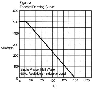
Admissable Power Dissipation - MilliWatts versus Ambient Temperature  $-^{\rm O}{\rm C}$
